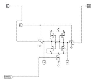
Figure 3.2 7-T SRAM cell
