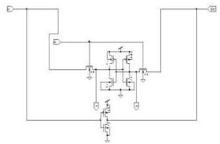
Figure 3.3 8-T SRAM cell
