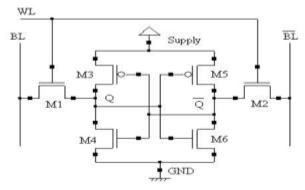
Figure 1.1 Conventional 6T SRAM Cell [1]
