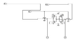
Figure 3.1 6-T SRAM cell
